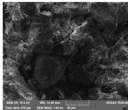
Figure 3. The SEM images of recycled refractory brick
