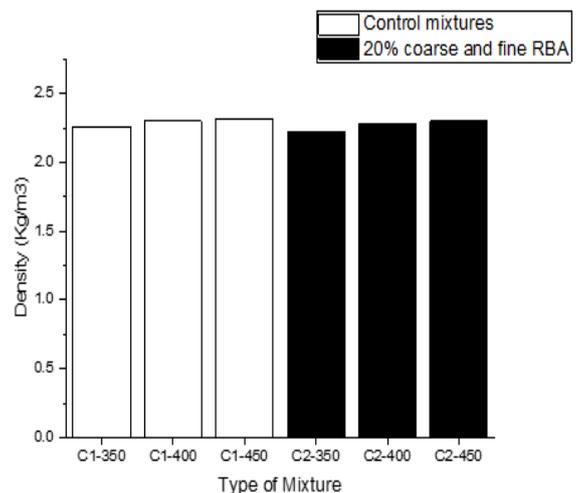
Figure 5. Effect of coarse and fine RBA on density.
