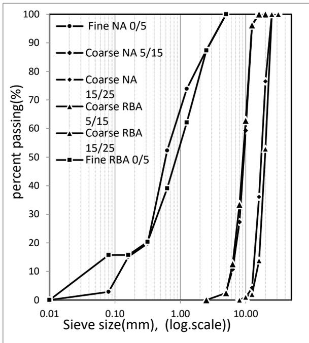
Figure 2. The grain size distribution for the natural and recycled refractory brick aggregates.
