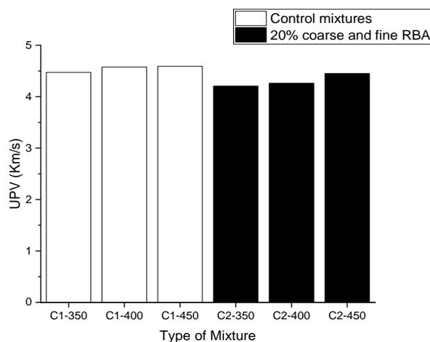
**Figure 6.** Effect of coarse and fine RBA on UPV.
