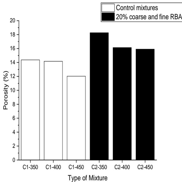
Figure 4. Effect of coarse and fine RBA on porosity.
