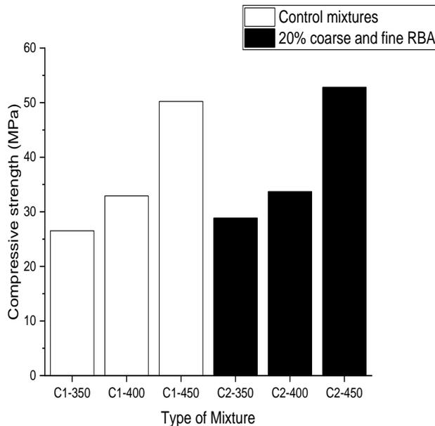
**Figure 7.** Effect of coarse and fine RBA on compressive strength.
