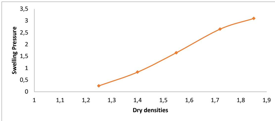
Figure 3: Swelling results at different initial dry densities at constant initial water content (w=0%)
