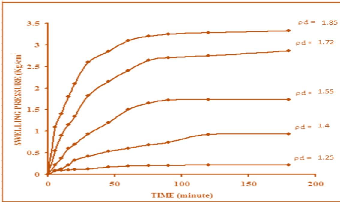
Table 2 shows the swelling results at different initial dry densities at constant initial water content ( $w=0\%$ )
