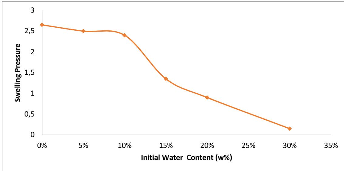
Figure 4 :swelling pressure at different initial water content for constant dry density  $\rho_d=1.72\text{gm/cm}^2$
